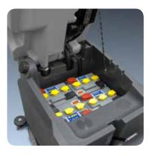
Great working autonomy thanks to the possibility to use 4 batteries 6 V 240 Ah granting continuous working up. Possibility to use also 2 batteries 12V. Less battery consumption thanks to rear wheeldrive. Large load tanks made of shock and acid proof polyethylene (real load of 75 l.), avoiding frequent stop for refilling.
